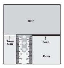
**Figure 1** Feet set at 3mm above the floor
